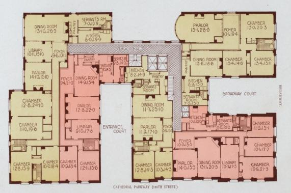
TYPICAL FLOOR PLAN OF ADDITION TO THE HENDRIK HUDSON APARTMENTS.
